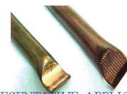
US welding copper tubes 0,8mm+0,8mm
