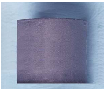
Element filtrant oxid aluminiu ( \phi 45 mm, grosime perete 1 mm)
